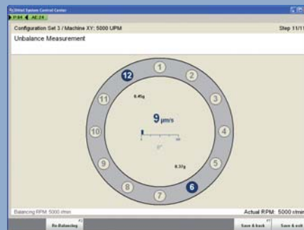
1 plane balancing (fixed position method)
