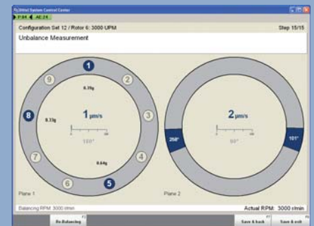
2 plane balancing (fixed position and spread angle method)
