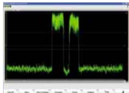
AE signals arising during dressing detected via AE fluid sensor
